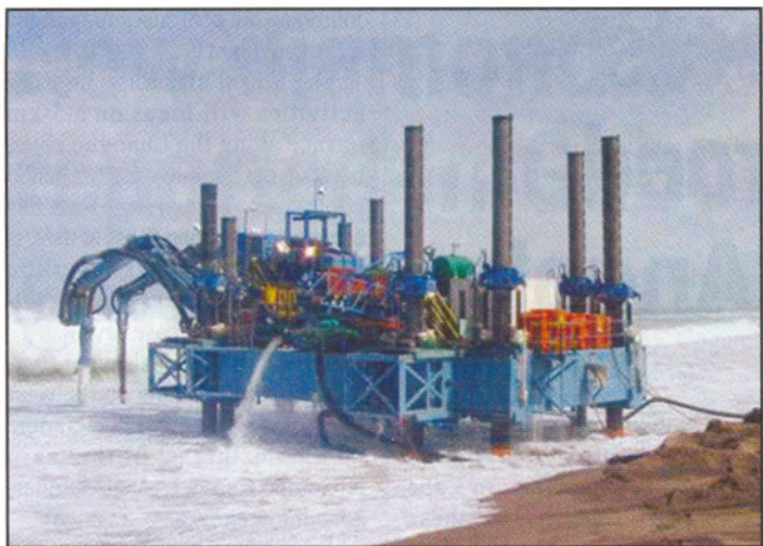
JETRIG JetRig during sampling operations in the ITC
