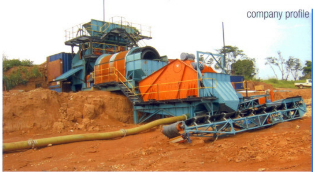
A 150 t/h alluvial plant erected and commissioned for 'Projecto Fucauma' in Angola in mid-2005. Endiama, the Angolan state diamond-mining company, and South Africa's Trans Hex are the main stakeholders in the new mine which is located in the north-east of the country.
